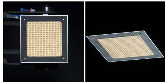
Figure 5: Sample holder with the PROPOSTE sample. The left image shows the frontal view ( \theta = 0^\circ , \phi = 0^\circ ); the right image shows ( \theta = 60^\circ , \phi = 342^\circ ). White point and border markers are visible.
