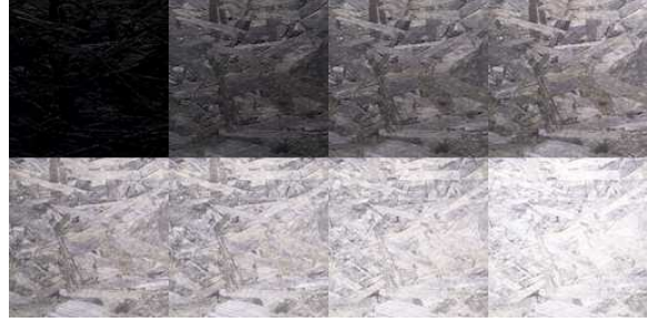
Figure 3: Shading Map . This set of images forms the shading map. In a shading map the average exit radiance is increasing linearly for every image.
