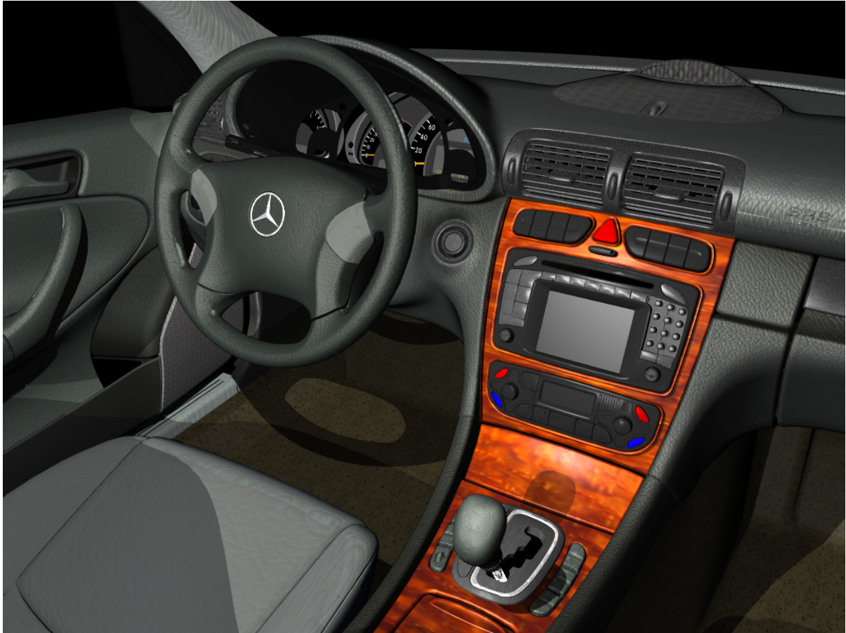
Figure 20: Visualization of the interior of a Mercedes C class using measured BTFs. This image was rendered using the OpenRT real-time ray-tracing engine [WBS02].
